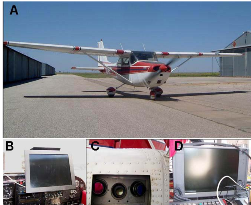
Figure 25. Components of TTAMRSS. (A) Cessna Skyhawk aircraft; (B) System monitor; (C) View of underside of aircraft showing cameras; (D) Computer.
