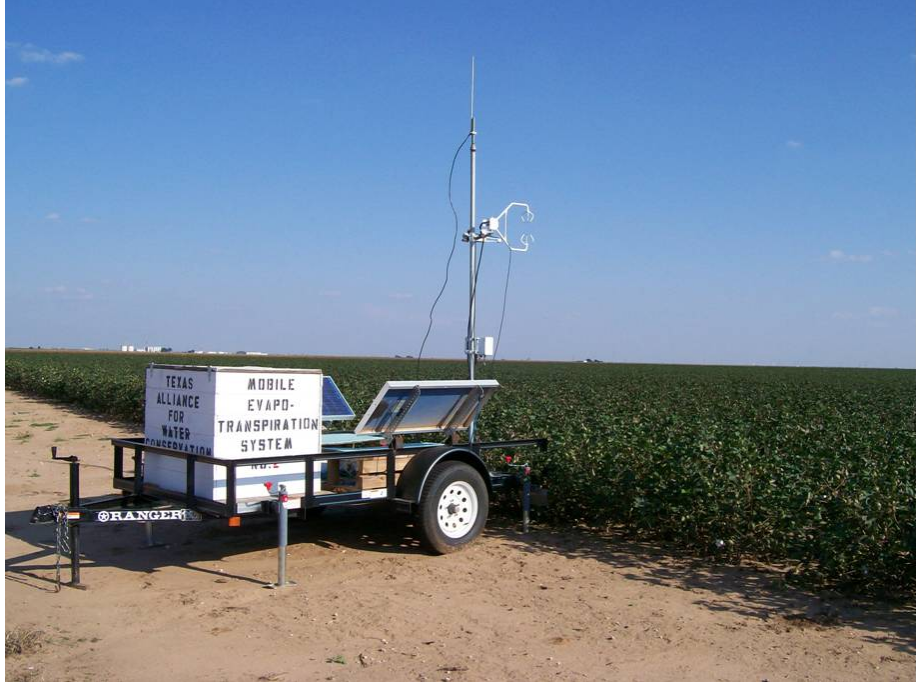
Figure 40. Mobile eddy covariance system located at Field 2.
