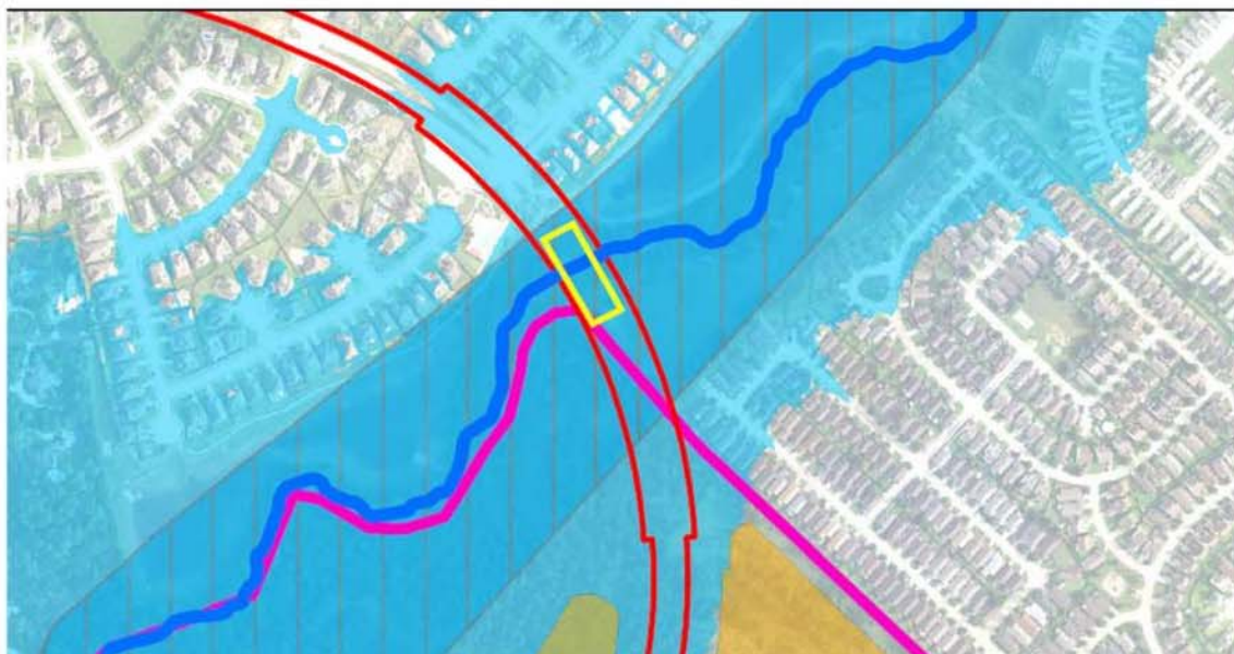
Figure 2. Proposed Bridge/Roadway and Floodway/Floodplain Hatched area - effective FEMA floodway; Blue shading - 100-yr floodplain draft SJTWS 1D-unsteady HEC-RAS with 2018 LIDAR and Atlas-14 rainfall
