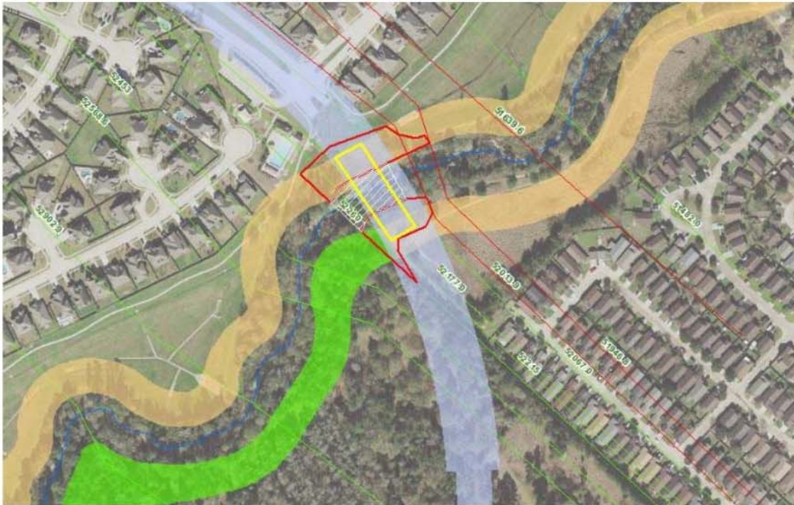
Figure 1. Proposed Bridge/Roadway and Selective Clearing Yellow outline – Proposed bridge; Hatched area - proposed concrete lining; Red outline - Proposed clearing and grubbing; Green shading - Proposed selective clearing; Red cross sections - higher 10-yr and 100-yr WSEL
