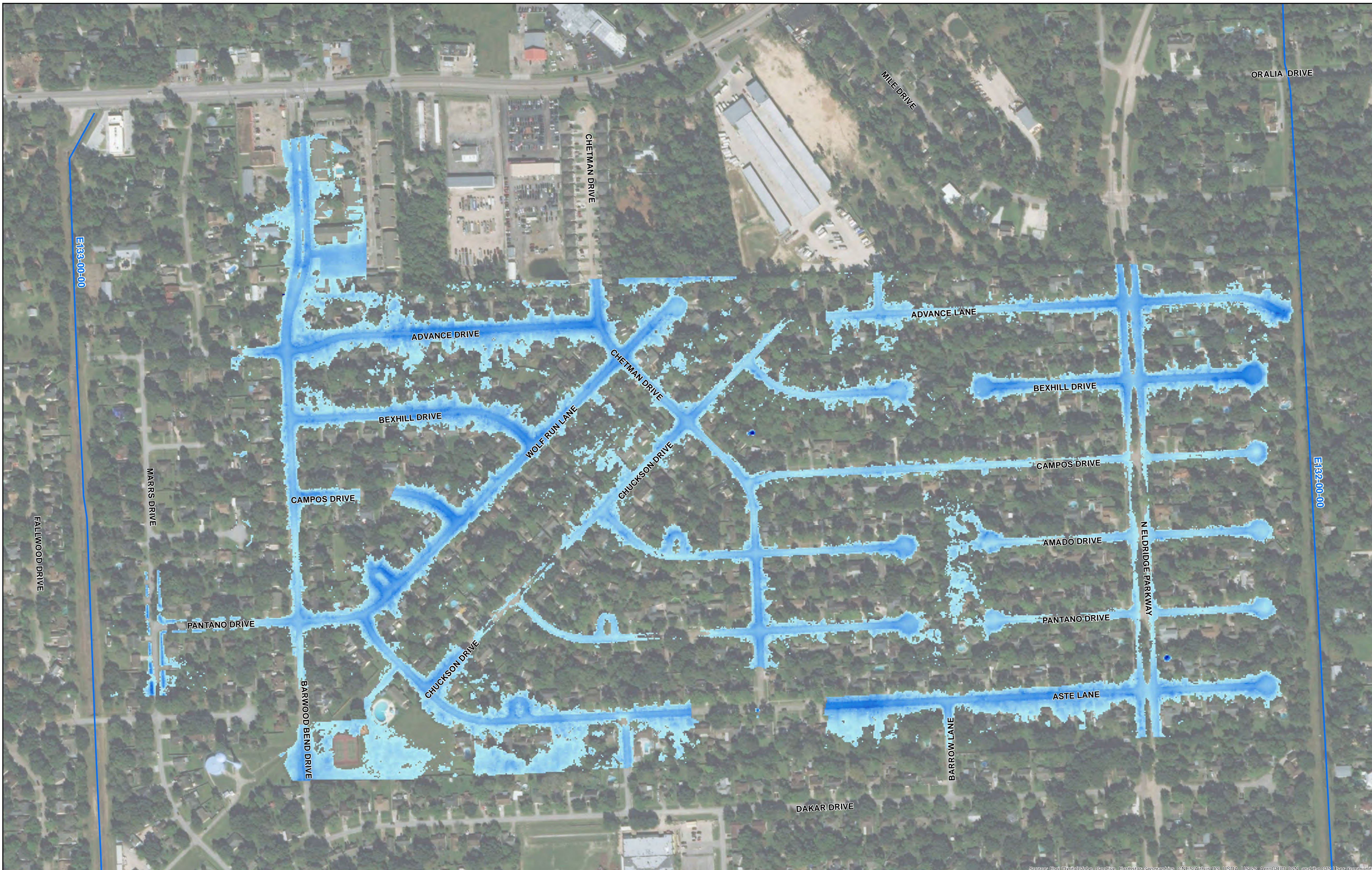
EXHIBIT 6 EXISTING PONDING RESULTS 10-YEAR STORM EVENT
