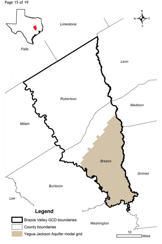
FIGURE 4: AREA OF THE GROUNDWATER AVAILABILITY MODEL FOR THE YEGUA-JACKSON AQUIFER FROM WHICH THE INFORMATION IN TABLE 4 WAS EXTRACTED (THE YEGUA-JACKSON AQUIFER EXTENT WITHIN THE DISTRICT BOUNDARY).
