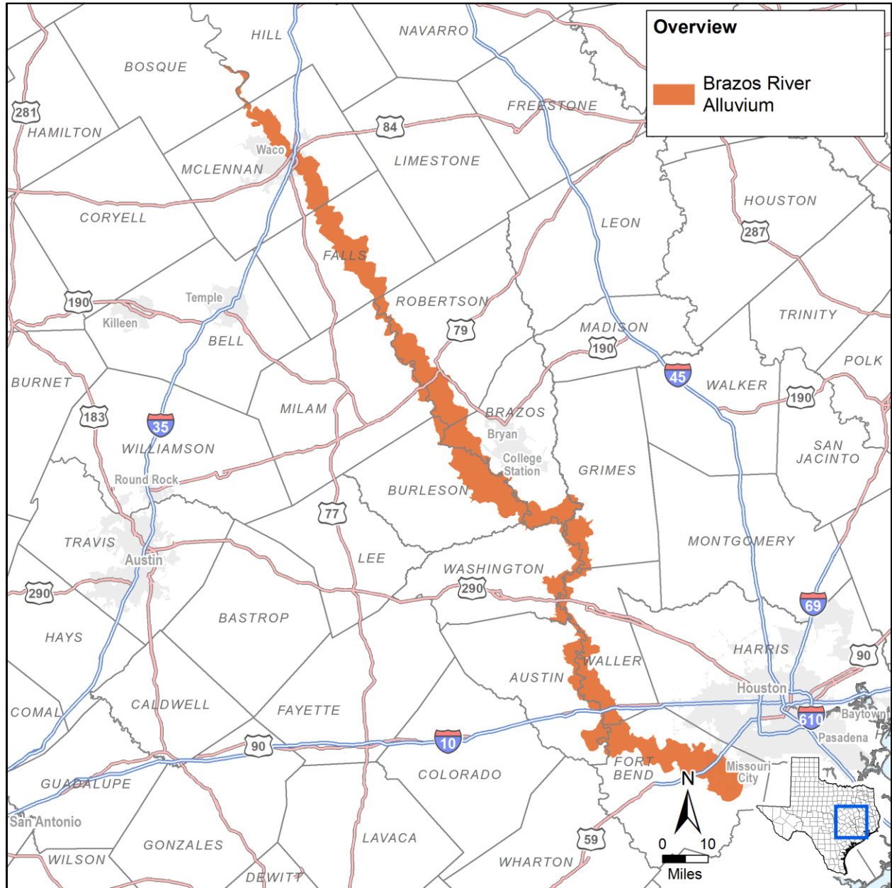
Figure 4.65. Brazos River Alluvium Aquifer extent.
