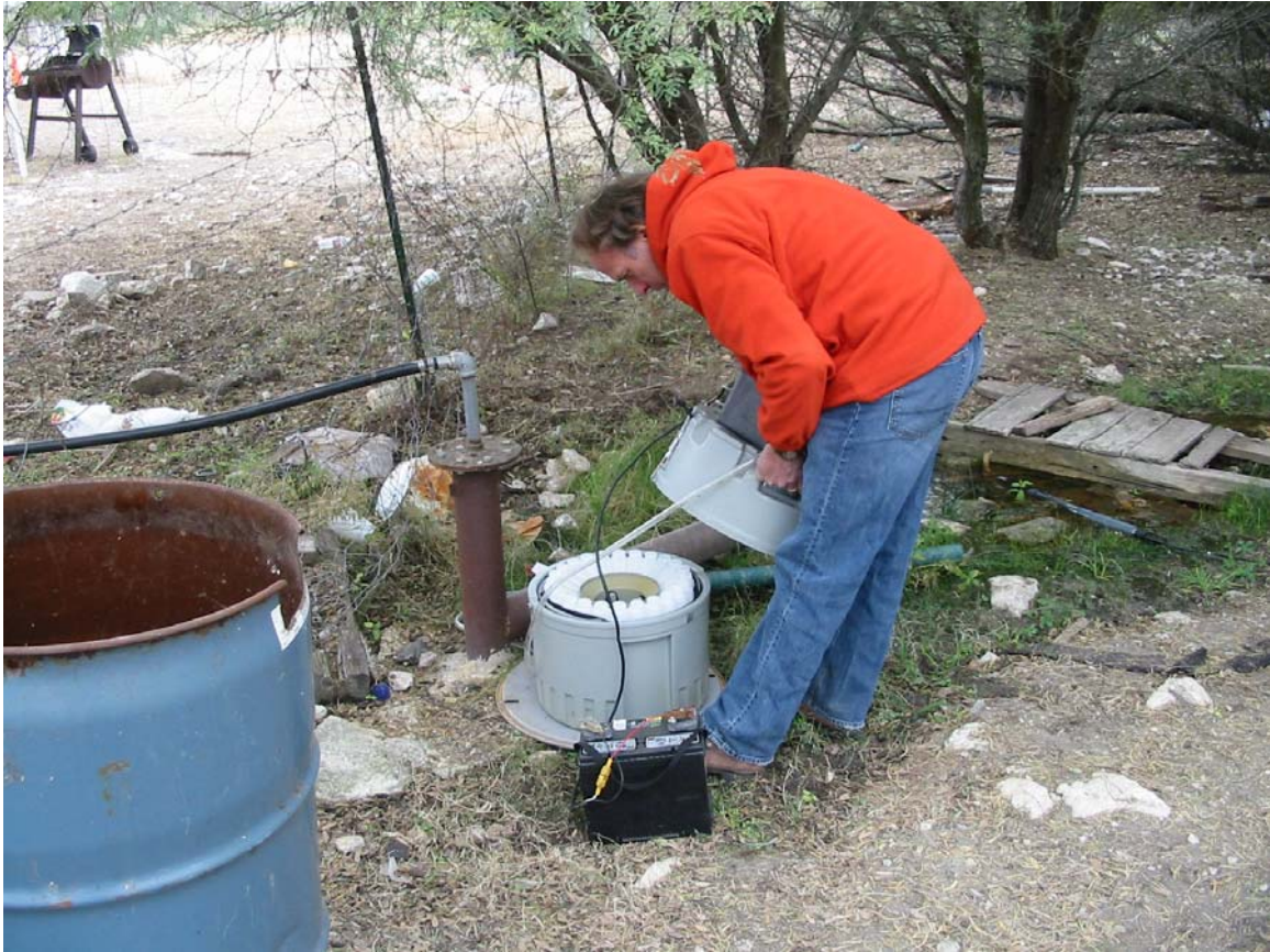
Figure 4.1. ISCO Automated Sampler Utilized in Study
