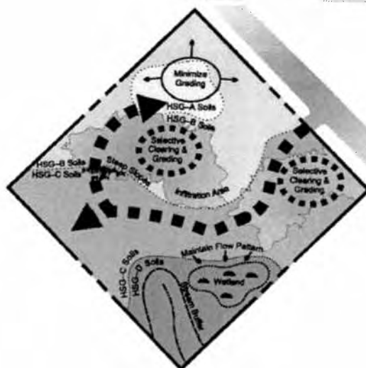
Figure 1.3.2-12 Guiding Development to Less Sensitive Areas of a Site (Source: Prince George's County, MD, 1999)
