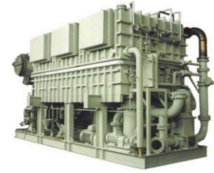
Example of a multi-stage flash evaporator used for desalination.
