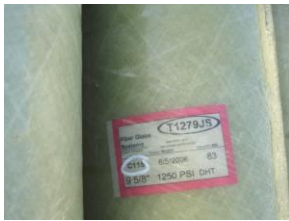
Fiberglass column pipe originally used for the production well, North Cameron Regional Water Project, August 2006.
