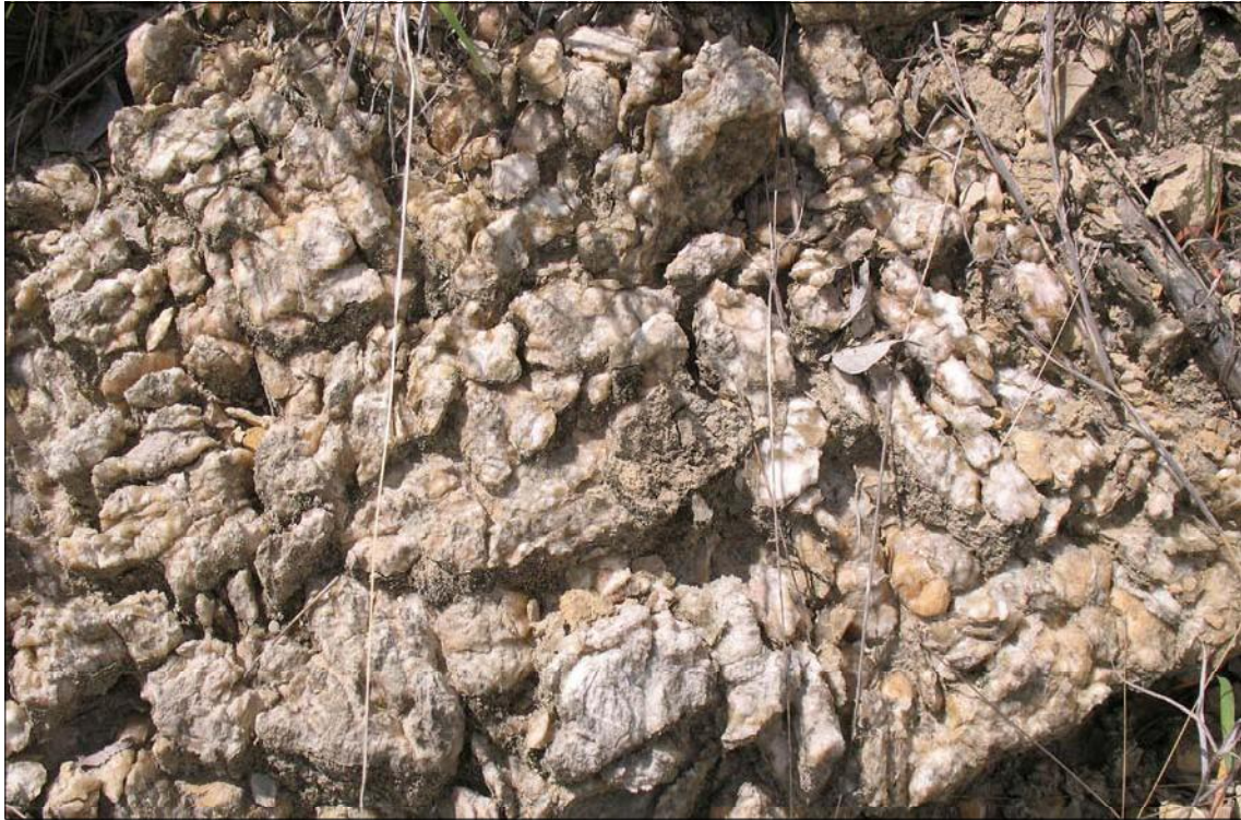
Closeup of Weathered Gypsum bed in outcrop located at approximately 1/4 mile Northwest of proposed dam alignment
