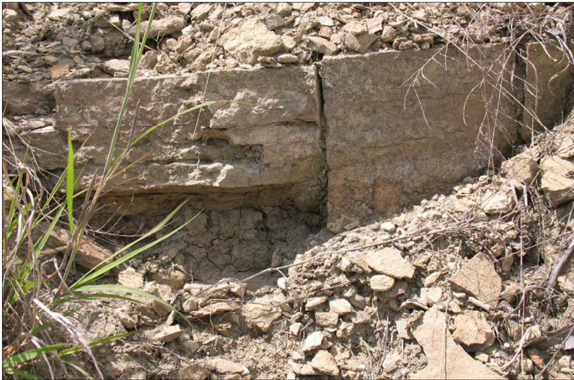
Vertical Fractures (Joints) in Limestone bed in outcrop located at approximately 1/4 mile Northwest of proposed dam alignment
