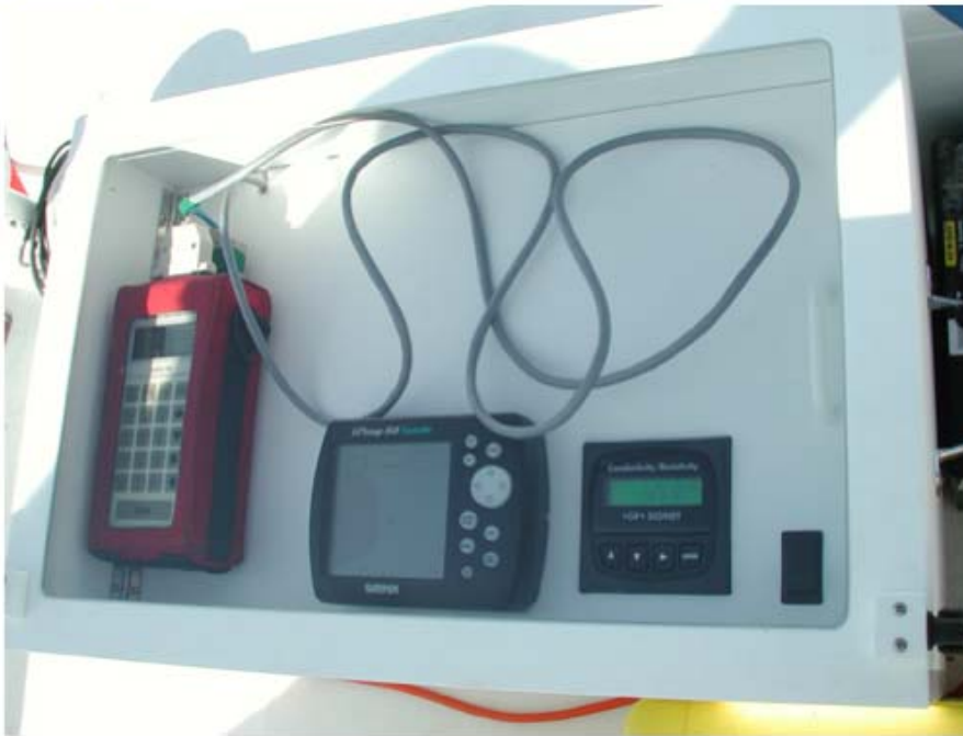
Figure A31: Photos of Dataflow operation in San Antonio Bay. The upper image shows the regulator pump box attached to the intake ram (right), the de-bubbler (near engine), and inflow pump to the Dataflow box (left). The bottom image shows the GPS, temperature, and conductivity displays as well as the datalogger (on left). All other sensors are in the lower level of the box.
