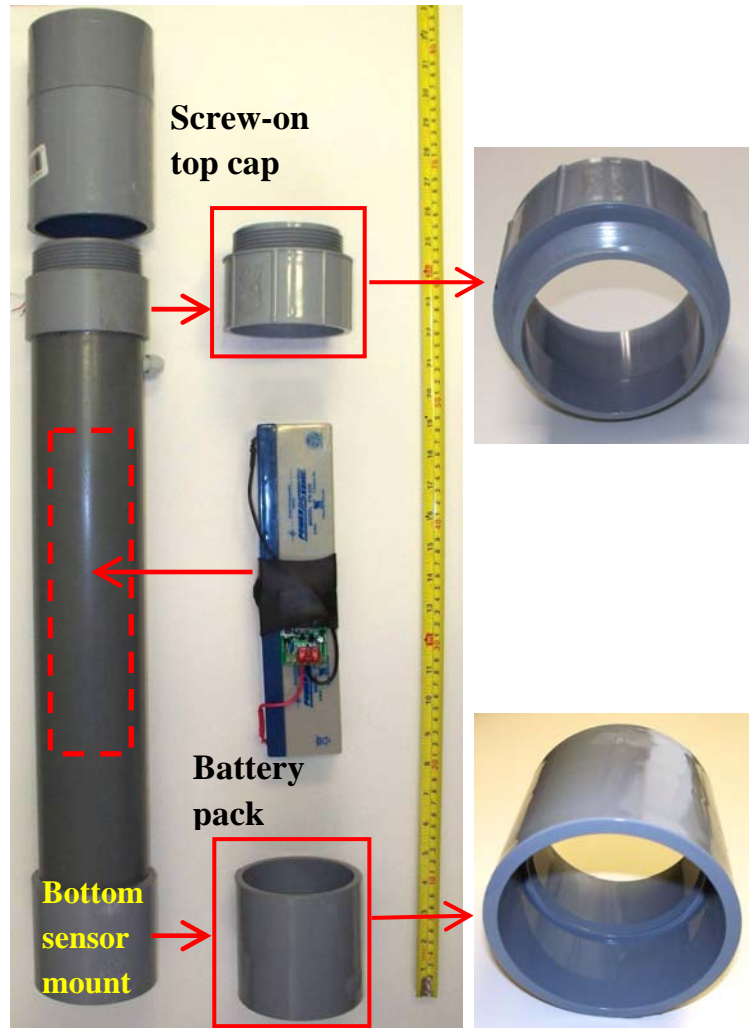
Figure 9. Main body of enclosure showing the male threaded/slip connector for the top cap (top right) and the female slip/slip connector for the bottom sensor (bottom right)
