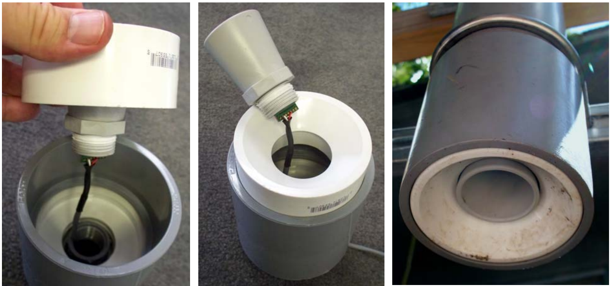
Figure 20. Final assembly of water level sensor with surround ring (left and middle) into the 3 inch female slip connector (right).
