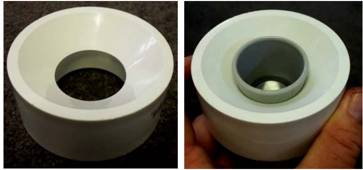
Figure 19. Sensor surround ring (left) with sensor (right)
