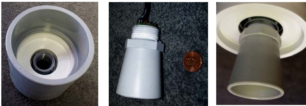
Figure 18. The assembly in figure 17 mounted in the 3 inch female/female connector (left), showing the 3/4 inch threaded socket into which the sensor (middle) screws, as shown (right).
