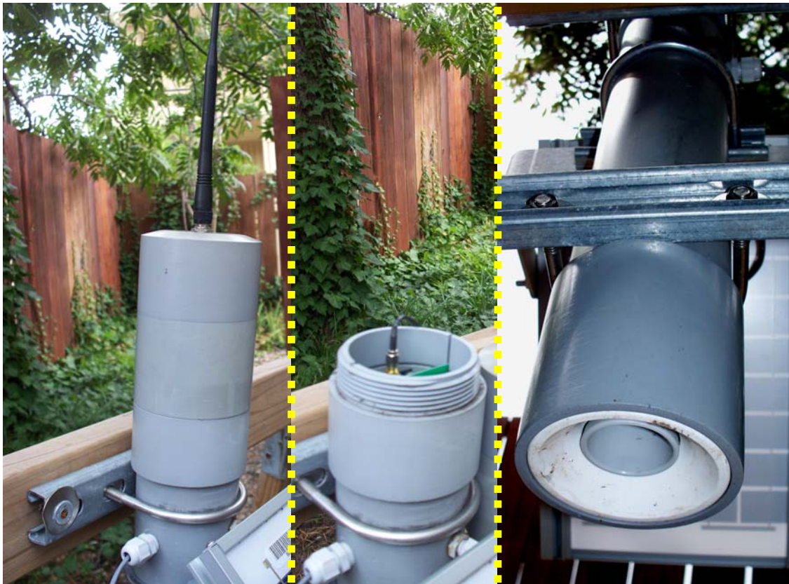
Figure 3. LCRTU showing top with antenna (left), top with screw-on cap removed (center) and bottom with downward facing acoustic water level sensor (right).
