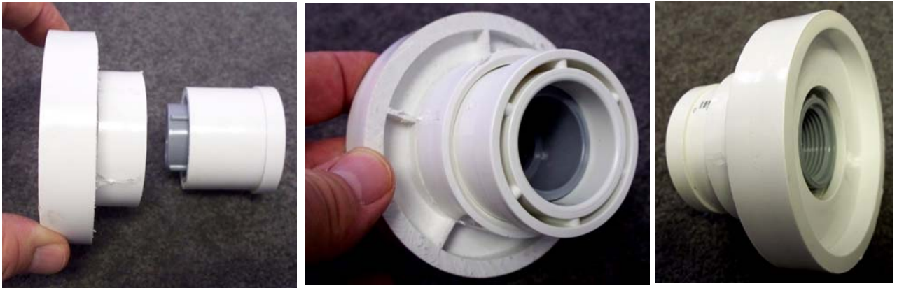
Figure 17. The assembly shown in figure 16 solvent welded to the modified 3 inch to 1 1/2 inch reducing bushing shown in figure 13 to create the sensor mount.
