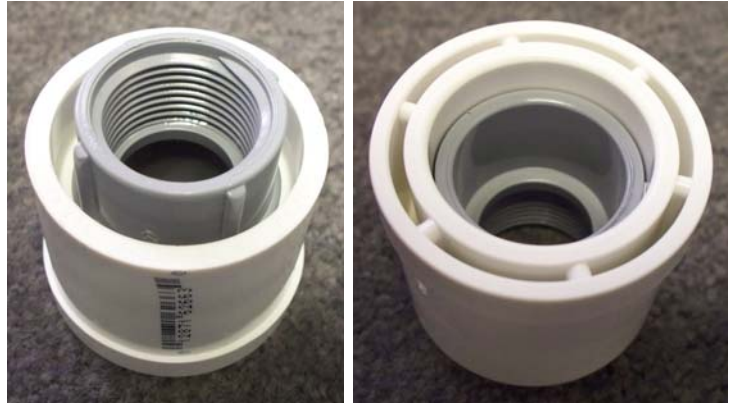
Figure 16. 1 inch slip to 3/4 inch female threaded adapter solvent welded to modified 1 1/2 inch to 1 inch reducing bushing,
