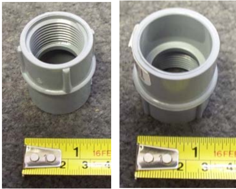
Figure 15. Views of threaded (left) and slip (right) ends of 1 inch slip to 3/4 inch female threaded adapter.
