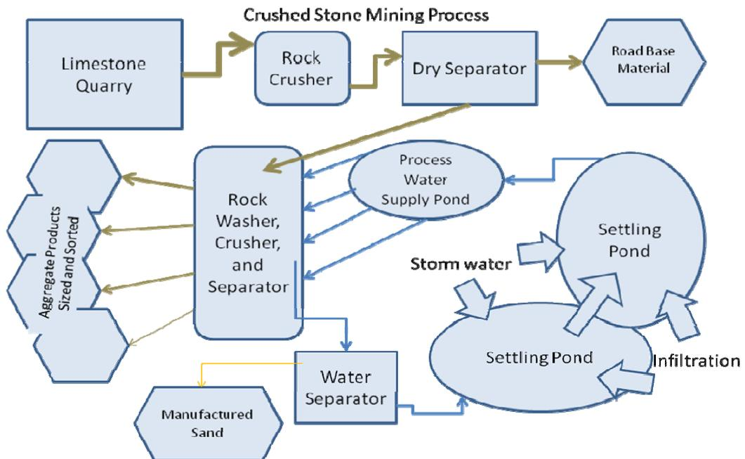
Figure 102. Flow diagram of typical crushed-stone process
