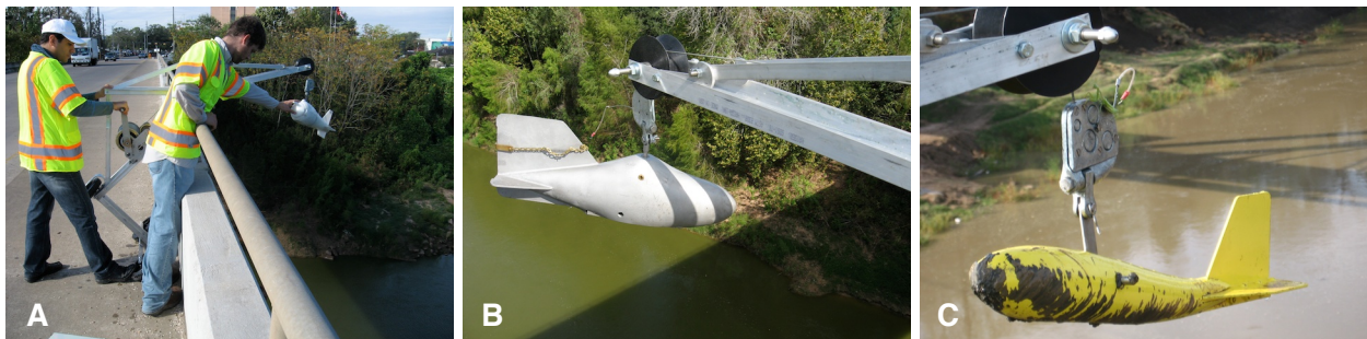
Figure 3.3: Primary sampling equipment. (A) US DH-2TM bag-type sampler suspended from the sampling crane; (B) US BMH-60 bed material sampler; and (C) sounding weight.
