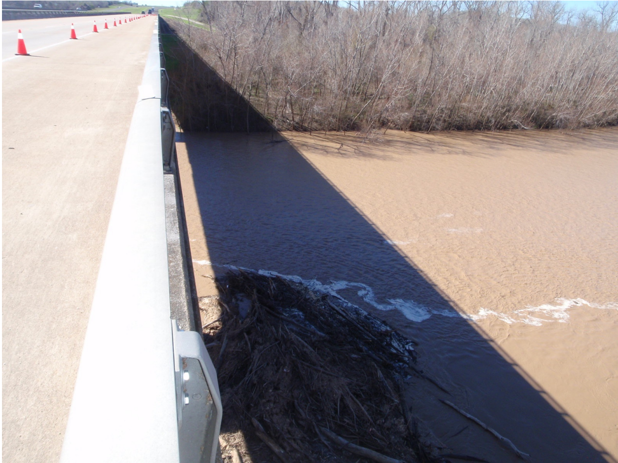
Figure 5.7: The Brazos River at the Hempstead station on January 27, 2012. The picture was taken in the afternoon at a flow rate of Q = 16,000 cfs, which was approximately equal to the effective discharge (table 5.4). The measurements made at this time were done during the rising limb of the event hydrograph. Measured concentrations on this day were the highest of any observed at Hempstead (wash load was 97%).
