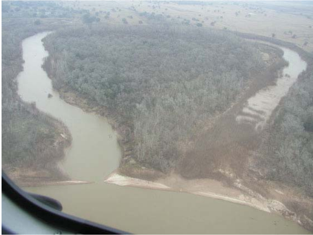
Figure 3.28 – Formation of Hog Island Oxbow – January 23, 2002. Gently sloping sand banks separate the south arm (right) from the Brazos River (bottom). Sand bar is beginning to form on the north arm and the connection channel is prevalent. Brazos River Flow ~4,800 cfs.
