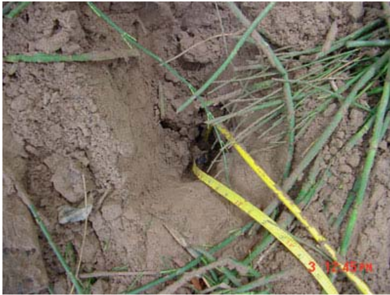
Figure 3.35 – Sediment Deposition on the banks of the Brazos River from December 2003 until June 2004. Over 12” of sediment was deposited on installed equipment.
