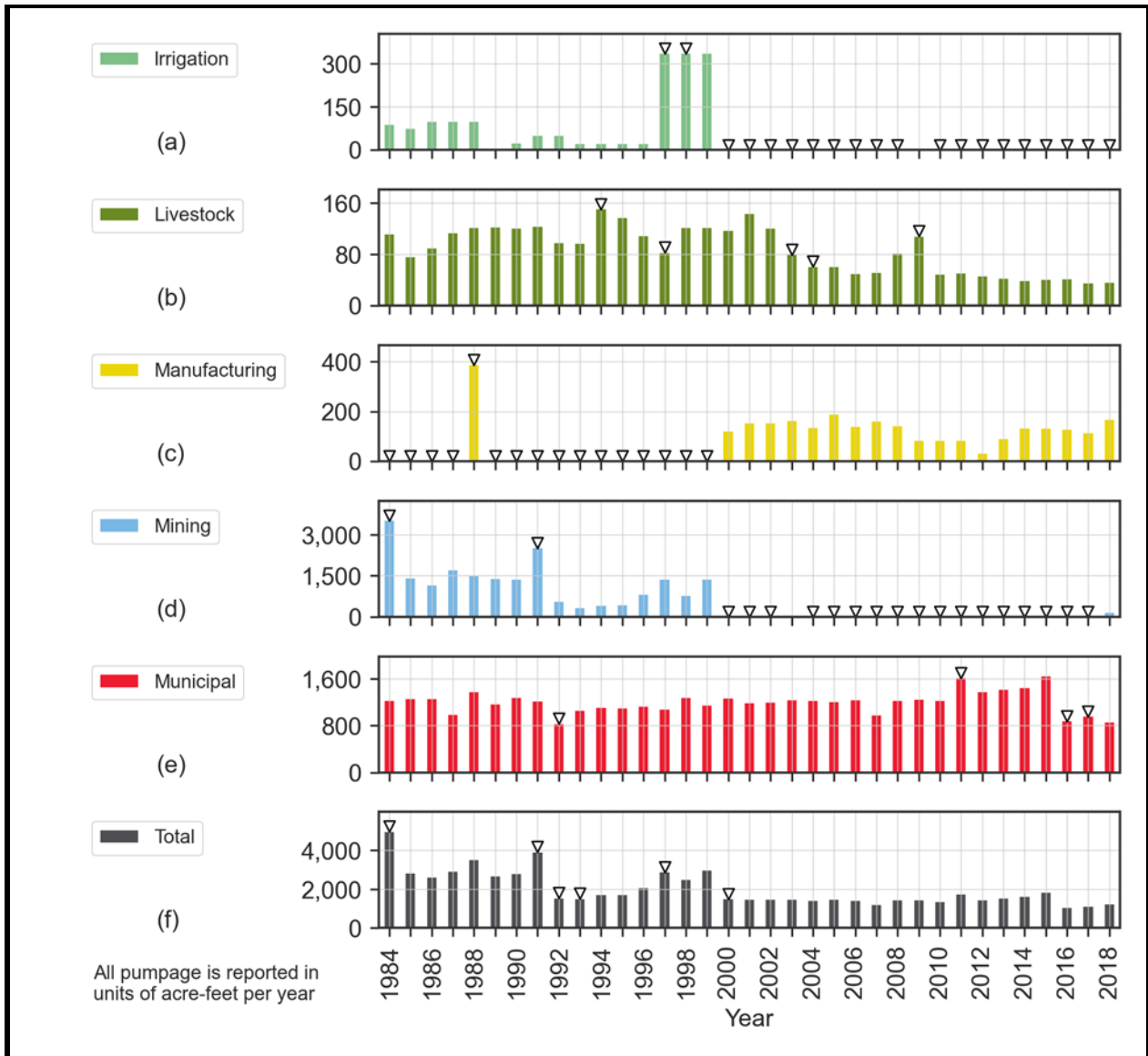
Figure 90. Crane County Pecos Valley Aquifer apparent anomalies based on the criterion of 1.5 standard deviations from the 3-year average of groundwater pumping in acre-feet per year as reported in the TWDB Water Use Survey data. Triangles mark years where the data appears anomalous.
