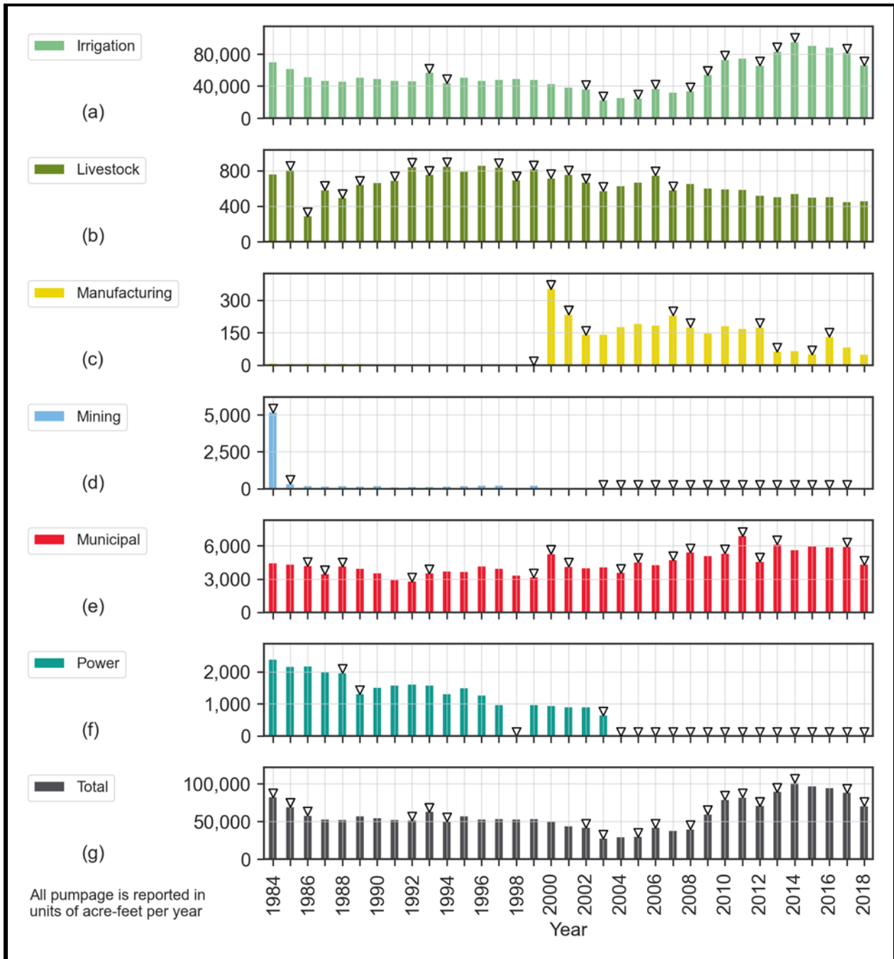
Figure 238. Pecos County Edwards-Trinity (Plateau) Aquifer apparent anomalies based on the year-to-year change in groundwater pumping in acre-feet per year as reported in the TWDB Water Use Survey data. Triangles mark years where the data appears anomalous.
