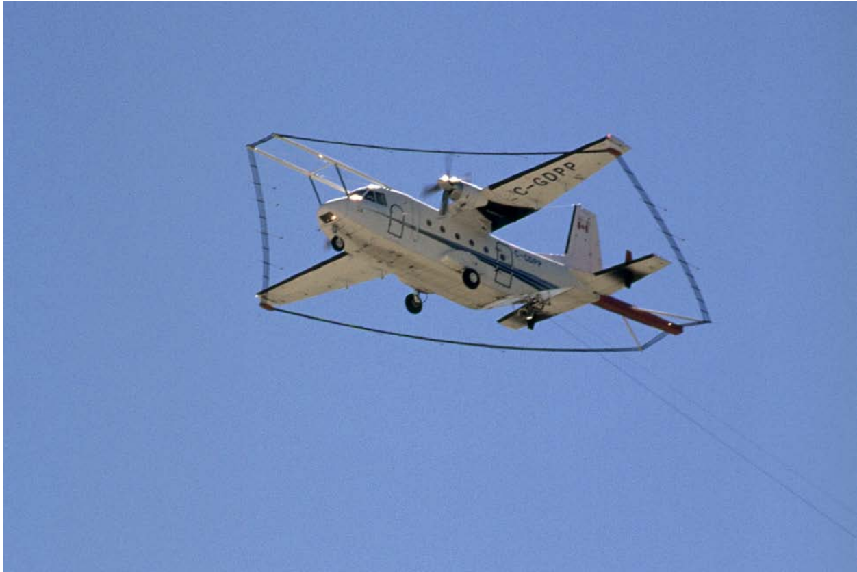
Figure 13. Geoterrex's GEOTEM airborne TDEM system operating over the Faysville study area, October 21, 1999. The six-turn transmitter loop is attached to the wing tips and booms at the front and rear of the aircraft. Cables trailing the aircraft tow the EM receiver and magnetometer (not shown). Photograph by David M. Stephens.
