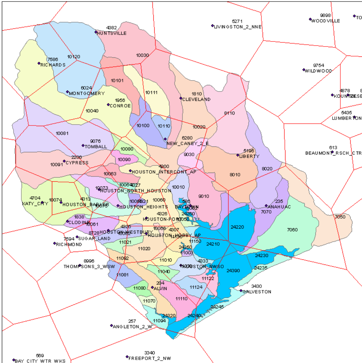
Figure 4. Rainfall stations (◆) and Thiessen polygons (red lines) used to estimate direct precipitation onto the Trinity-San Jacinto Estuary.
