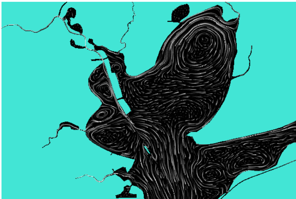
Figure 7.4 Residual flow pattern for the no power case, Compare the flow traces in Dickinson Bay and the cooling pond near Trinity Bay with the ones for the existing condition (Figure 7.3)
