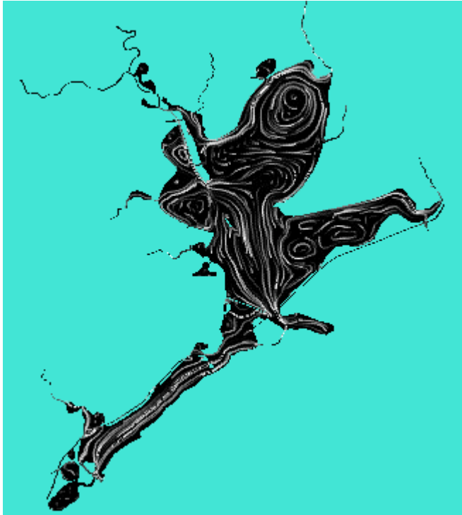
Figure 7.1 Residual flow pattern for the existing case
