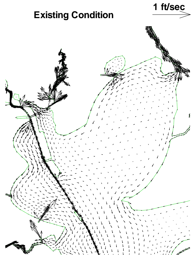
Figure 7.11 Residual vectors in mid and upper Galveston Bay for the existing condition; notice the vectors for the power plant operation
