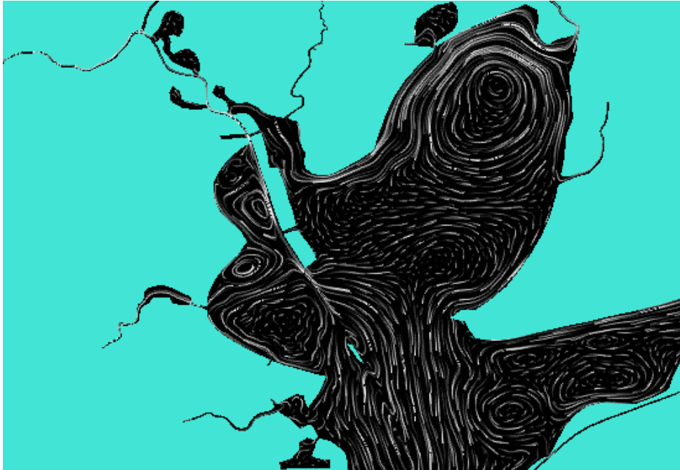
Figure 7.3 Residual flow pattern for the existing case in the mid and upper Galveston Bay; notice the influence of power plant intake and withdrawal
