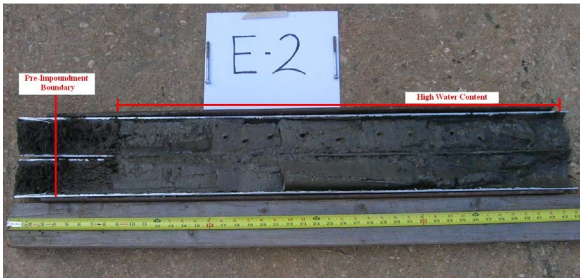
Figure D2 – Sediment Core E-2 from Eagle Mountain Lake, showing the pre-impoundment boundary 4 inches above the base of the core (left). The pre-impoundment boundary is marked by the change in soil structure below and above the area 4 inches up from the core base. Above 8.5 inches from the core base, the sediment moisture content is extremely high.
